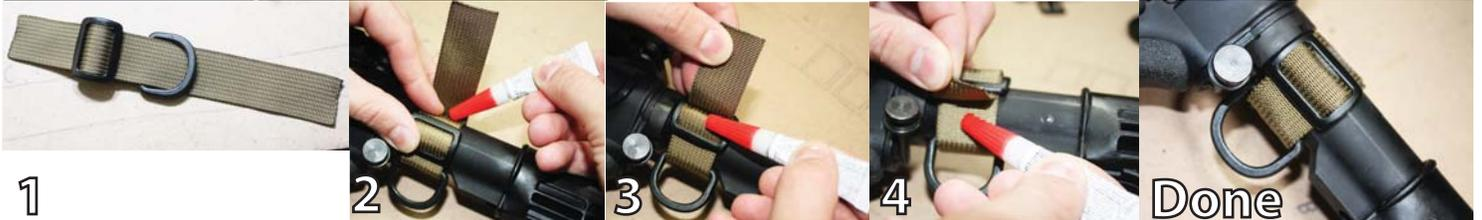
For Semi-Permanent attachment of the *Buffer Tube Sling Mount* use Superglue as illustrated above. If your Weapon System already has a rigid sling point at the rear of the receiver (recommended) or under the *Buffer Tube* then disregard. To prevent rotation, small amounts of Superglue can also be placed between the nylon and the *Buffer Tube*.
